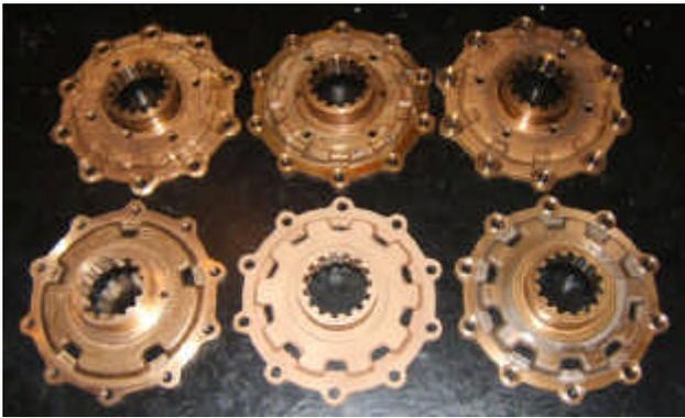
Six thrust plates done and ready to go back to work. The one on the lower left is a new one in the later Eaton style as opposed to the earlier Hall Scott type in the top row. Notice that they reduced the number of lubrication holes to try to get more strength.
