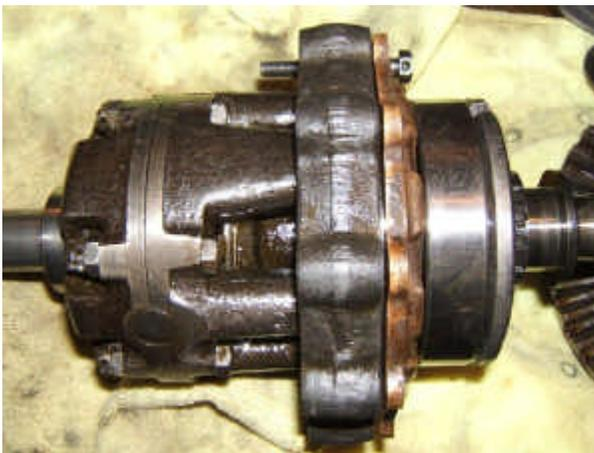
Assembled except for the ring gear and housing. The mechanism fits into the "bell housing" and the ring gear fits over the bell, it all bolts together and goes in the differential housing.
